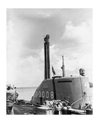
A submarine snorkel is a device that allows a submarine to operate submerged while still taking in air from above the surface. It was invented by the Dutch shortly before World War II and copied by the Germans during the war for use by U-Boats. Its common military name is snort.
